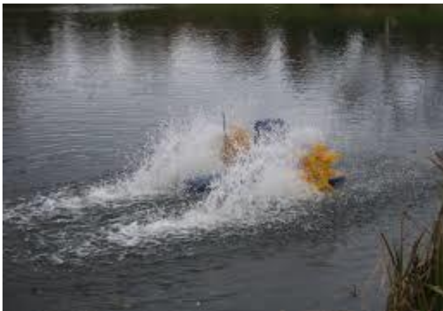
Floating Aerators with Cutter.
