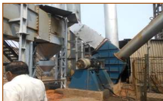
Fig No.6.10 (10) Centrifugal Blower of 90KW and 1440RPM, Capacity 40000m 3 /Hr, Stack height 35meters, Wet scrubbing system
