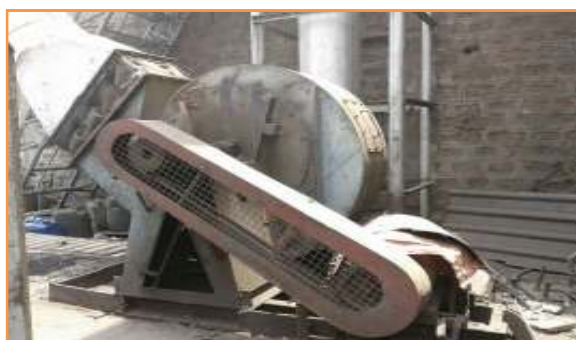
Fig No.6.10 (9) Centrifugal Blower of 75KW and Capacity of 30000m 3 /Hr, Stack height 35 meters, Wet scrubbing system
