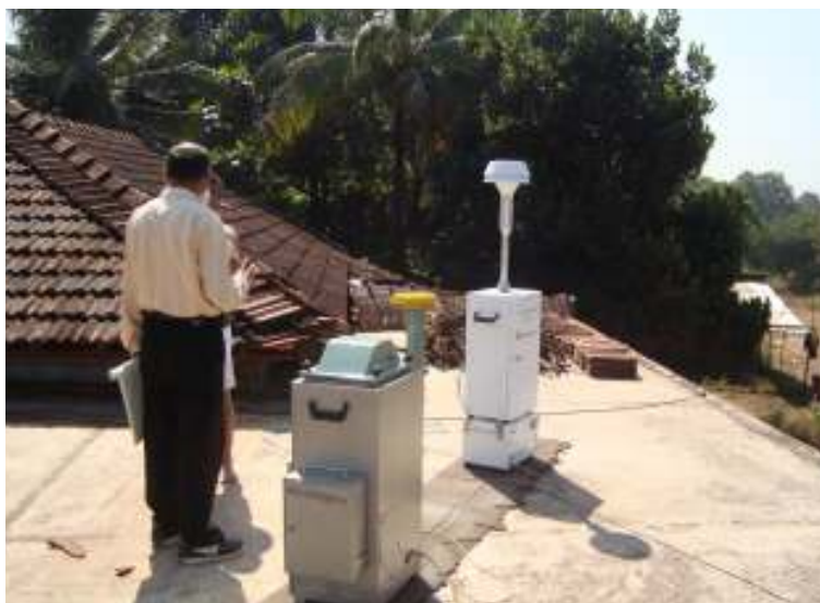
Plate – 3d: View of the PM10 and PM2.5 Samplers placed at the NAMP Monitoring Station at Amona, Goa.
