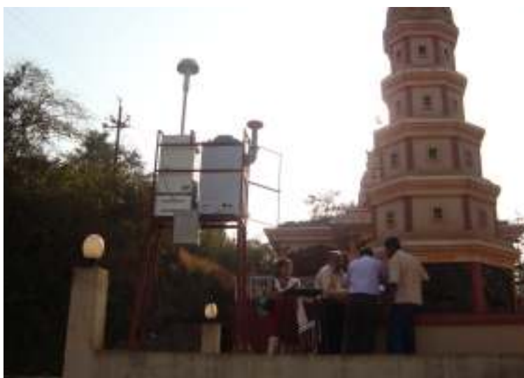
Plate – 3b: View of the PM10 and PM2.5 Samplers placed at the NAMP Monitoring Station at Honda – Sattari, Goa.
