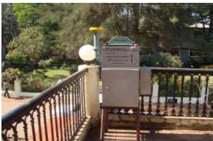
Plate – 3a: View of the PM 10 and PM 2.5 Samplers placed at the NAMP Monitoring Station at Bicholim, Goa.
