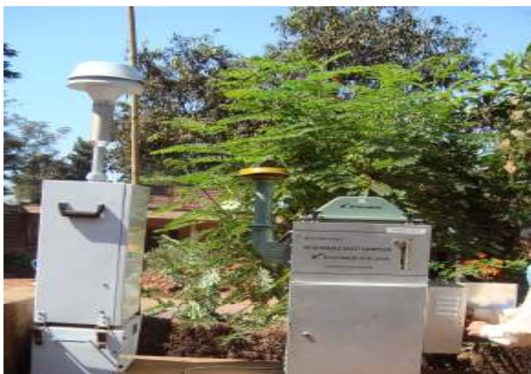
Plate – 3g: View of the PM 10 and PM 2.5 Samplers placed at the NAMP Monitoring Station at Usgao, Goa.
