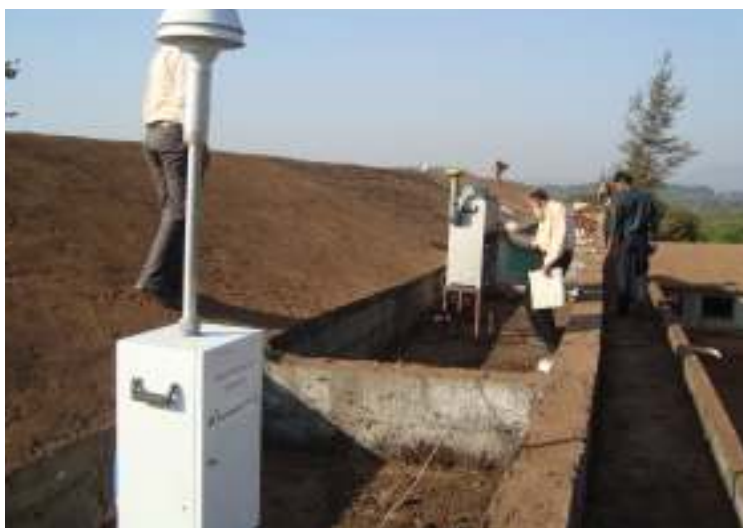
Plate – 3e: View of the PM10 and PM2.5 Samplers placed at the NAMP Monitoring Station at Codli, Goa.
