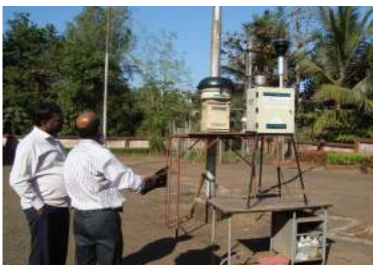
Plate – 3f: View of the PM10 and PM2.5 Samplers placed at the NAMP Monitoring Station at Curchorem, Goa.
