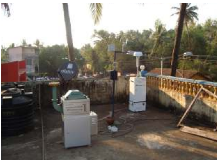
Plate – 3c: View of the PM10 and PM2.5 Samplers placed at the NAMP Monitoring Station at Assanora, Goa.
