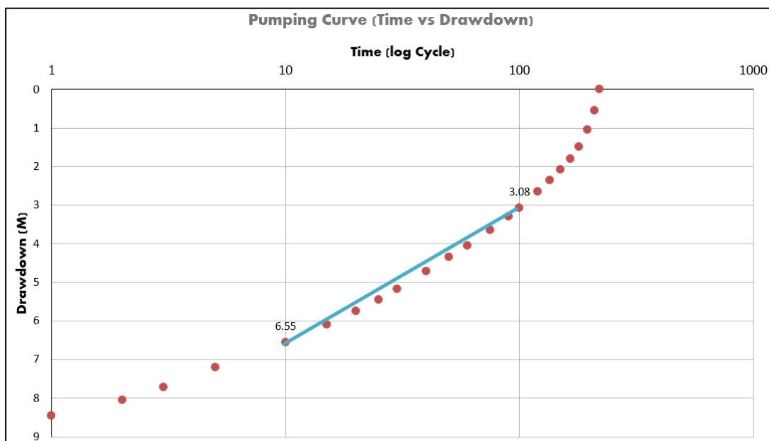
Figure 13 Log Time vs Residual Drawdown (Recovery Test – Jacob Method)
